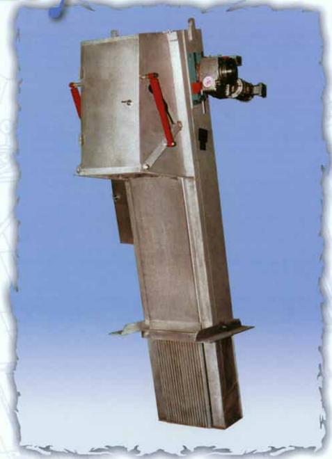
All bar screens are fully assembled and thoroughly shop tested to insure trouble-free operation prior to shipment. Units can be fabricated in sections to allow installation in existing structures.
