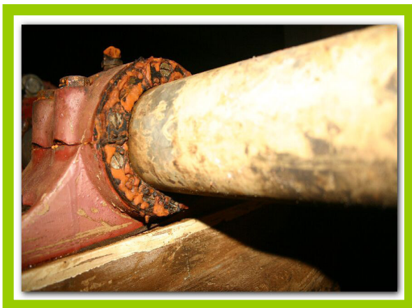
AFTER: Picture of AMWELL Greaseless Flocculator Bearing System at Racine, WI facility after 3 years of use
