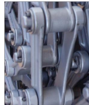
ABOVE: New DuraMax Cast Stainless Steel chain. Comparing new chain above to that installed in 2004, there is hardly a difference.
