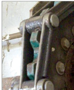
ABOVE: DuraMax Cast Stainless Steel chain installed in 2004 looks new; negligible maintenance since 2004 (photographed in 2010).
