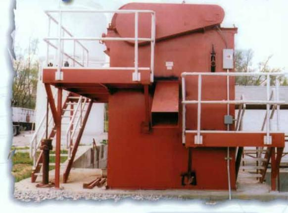
Four sizes of "dewatering screws" are available in systems offering capacities from 50 to 400 GPM, while our bucket elevator systems offer matching removal capacities. All systems can be timer controlled for automatic operation during peak flow periods.
