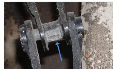
ABOVE: Plastic grit collector chain. Arrow indicates area where plastic is worn through
