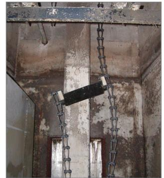
ABOVE: Broken plastic chain on grit collector
